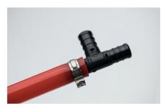
Step 3: Place PEX pinch clamp nub between tool jaws and ratchet the clamp until the PEX Pinch Clamp Tool auto-releases. This action will assure that the PEX pinch clamp is fully engaged.
