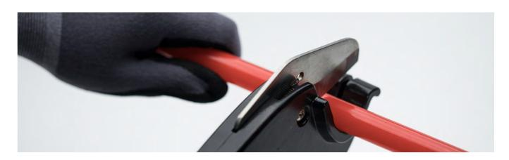
Step 1: Cut the pipe vertically and precisely with a pipe cutter
