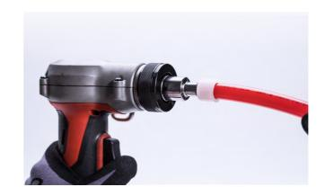
For electric pipe expansion tool, slide the pipe onto the end of the tool head until it stops. Press the button consistently to expand. Push the pipe at the meantime until it reaches the shoulder of the tool head.
