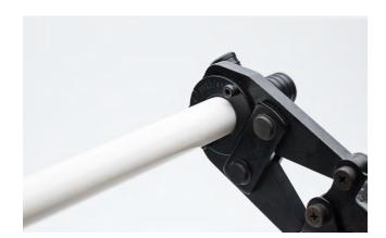
Step 3: Place the crimping end of tool around the crimp ring and press the handles together.
