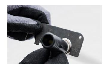
Step 4: Check for proper crimp with the Go/ No-Go gauge.
